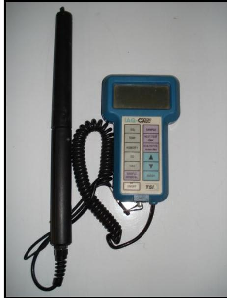
**Fig. (3-2): Mono and dioxide carbon (CO, CO<sub>2</sub>) concentrations measuring device**
