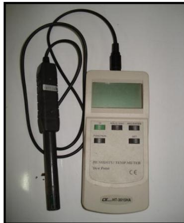
**Fig. (3-6): the device that was used for the measurements of air temperature and humidity**
