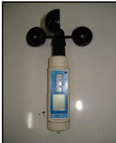
**Fig. (3-5): Anemometer device used for measuring wind speed.**
