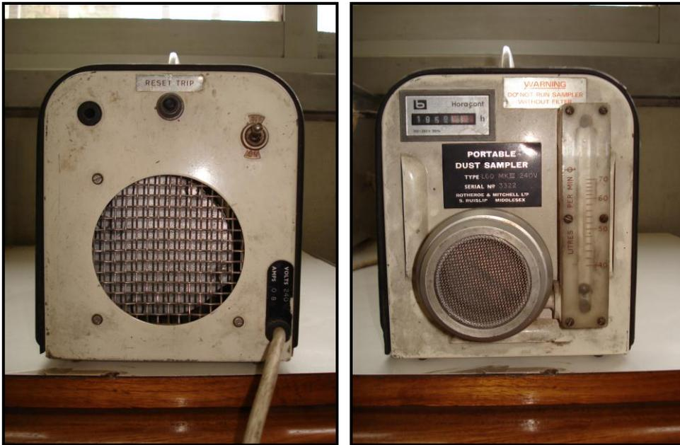
Fig. (3-4): Front and back view of Low Air Sampler (Sniffer) device features.
