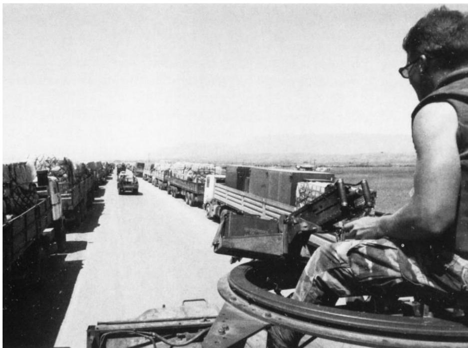
*Cpl Darryl F. Fuller of MSSG 24 mans a rig-mounted M-2 .50-caliber heavy machine gun atop a M-934 five-ton truck. This convoy carried bulk foods, building materials, and medical supplies to Refugee Camp 1 at Zakho.*
