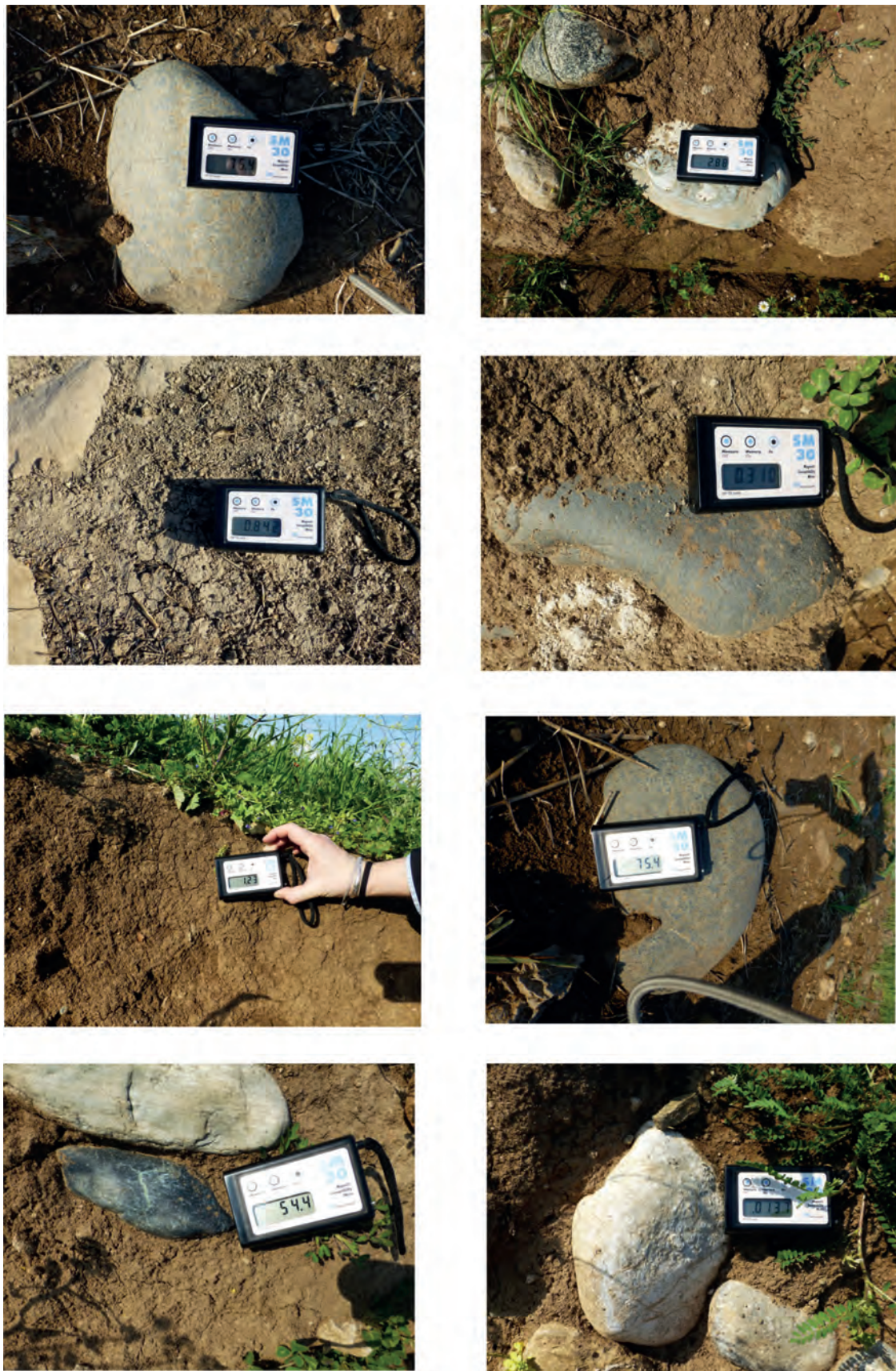
Fig. B4.1: In situ magnetic susceptibility measurements taken for rock samples and soil profiles with a handheld Kappa meter (SM-30, ZHstruments) with a sensitivity of \pm 10^{-7} [SI-units]. Photos by Jörg Fassbinder.
