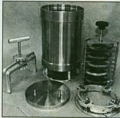
Figure (2-14) Pressure Aging Vessel (PAV) Equipment (Super-pave Fundamentals, 2010)
