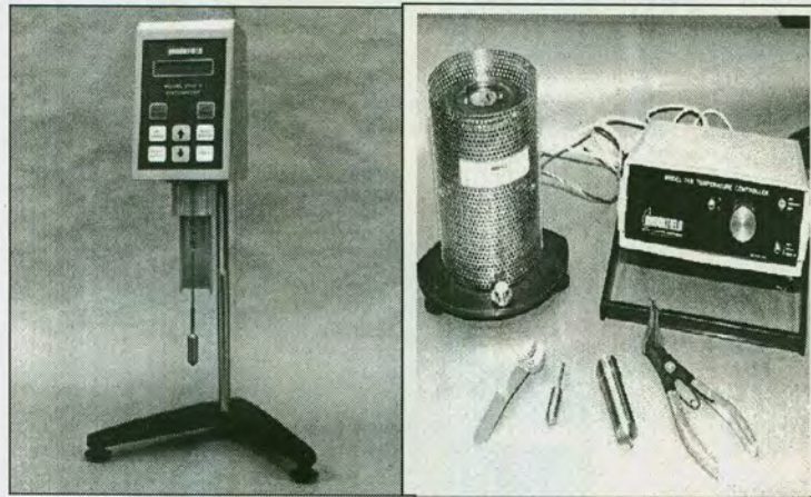
A-Rotational Viscometer Equipment.
