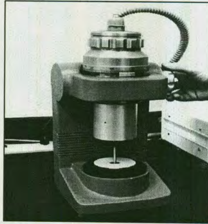
Figure (2-9) DSR Test Equipment
