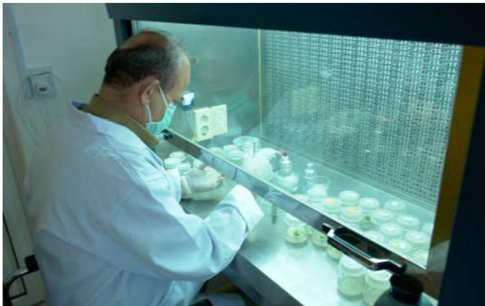
**Figure 8.** Laminar Air Flow Cabinet.
