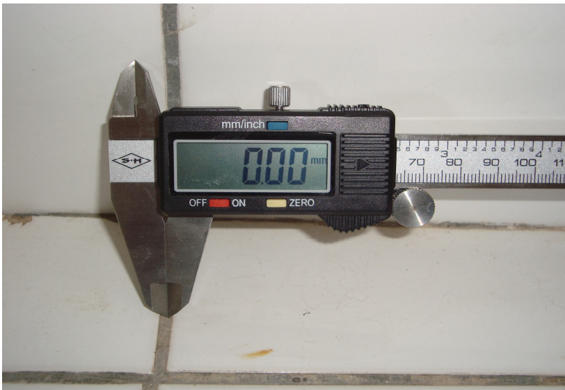
Figure (9): Vernier - Electronic digital caliper for measuring skin fold thickness in experimental rabbits.
