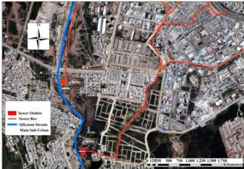
Fig.(1.1): The Locations of Two Sewage Outlets in the Study Area, Outlet 1 and 2 in Awabaraw Asha Spi 418 Sub-Districts, (Researcher)
