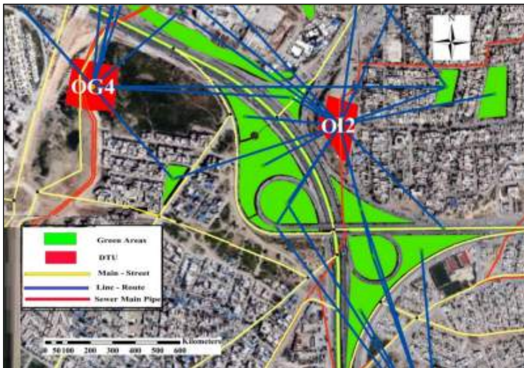
Fig.(5.4): The Results of the Network Analysis – OD Cost Matrix of Optimized Nominated Areas OI2 and OG4, (Researcher)
