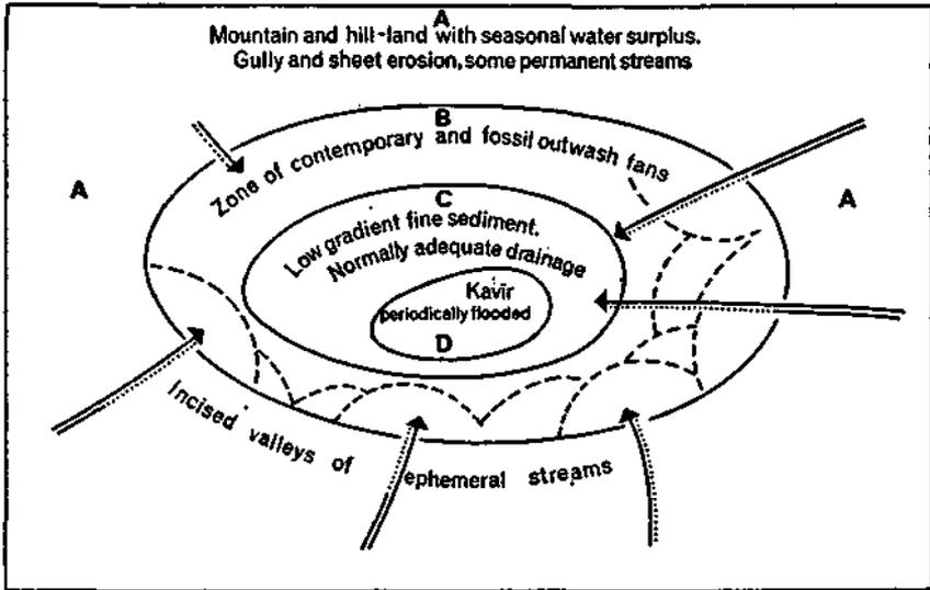
Fig. 138. Schematic plan of an Endoreic basin.
