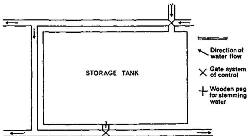
Fig. 148. Detail of irrigation scheme at Kāshif.
