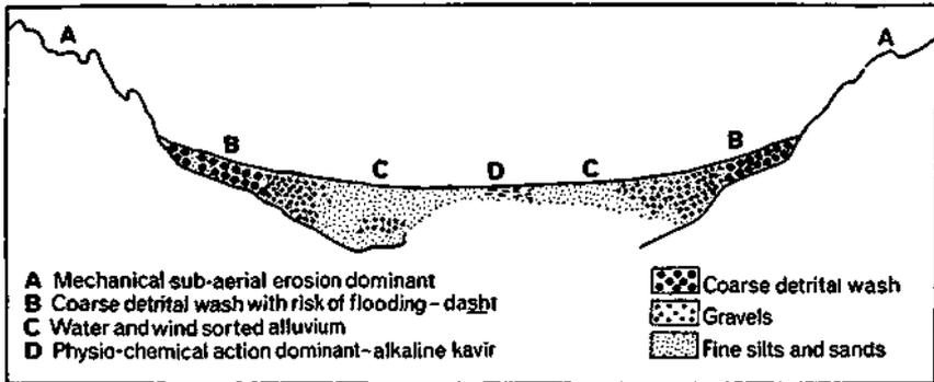
Fig. 137. Schematic section of an Endoreic basin.
