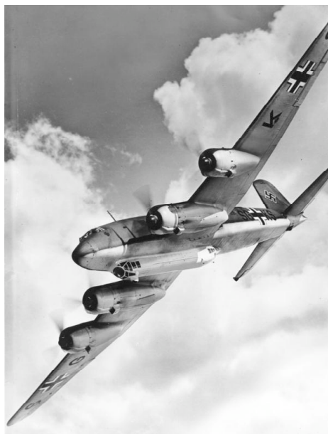
Figure 4-13. Focke-Wulf Fw 200 Condor. This is the long-range aircraft type used for Operation MAMMUT—designed as an airliner, it was one of the most aesthetically pleasing German aircraft ever built, but fraught with problems when used for cargo drops. Unlike the Junkers Ju 290 (Figure 4-14), which featured a rear slipway, the Condor had only a narrow side exit, which often caused problems when parachutists and cargo were to be ejected in rapid succession. (Photo courtesy of the Bundesarchiv [Bild 146-1978-043-02]).
