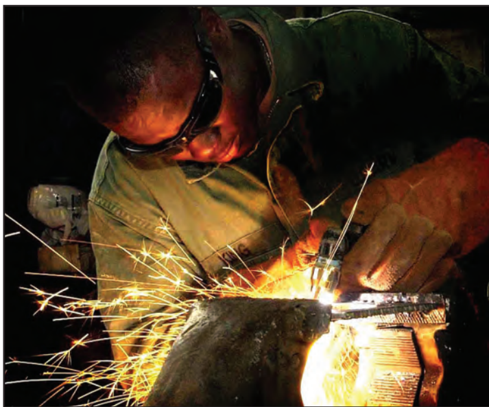
Figure 126. Sergeant Ariel King, from the Stryker Brigade Combat Team, 25th Infantry Division, welds a new antenna brace for a tactical vehicle in the brigade's Forward Maintenance Company shop at FOB Marez, Iraq.
