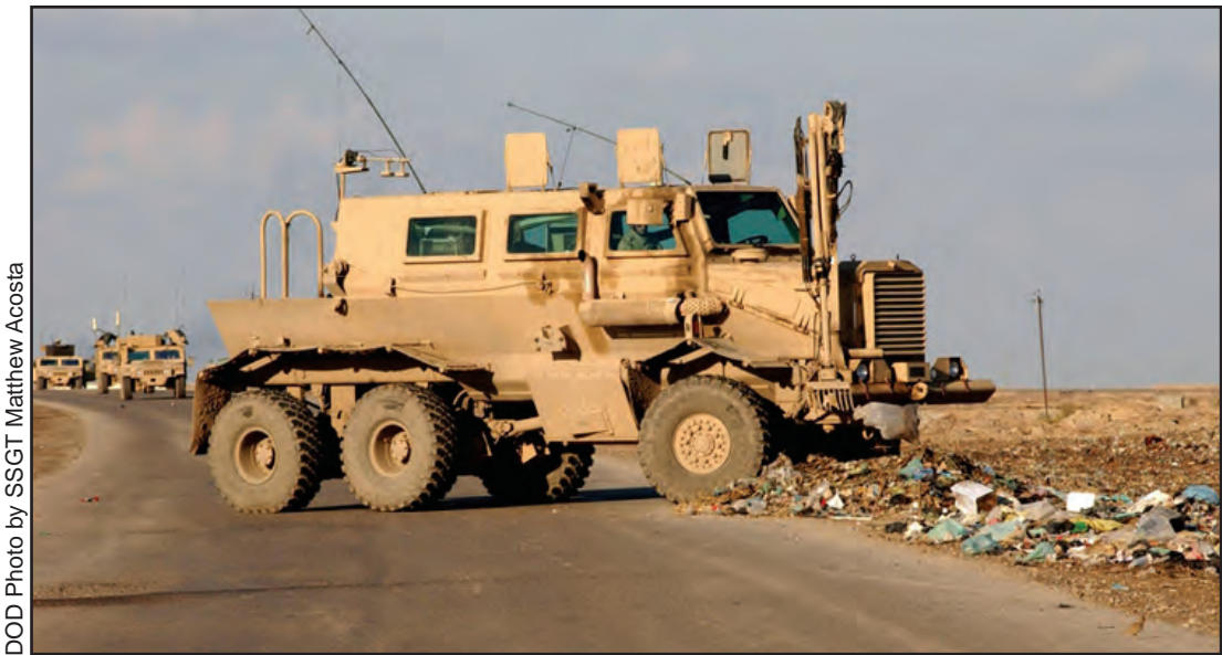
Figure 70. A Buffalo vehicle belonging to the Army Reserve's 467th Engineer Battalion uses its hydraulic arm to probe a trash pile thought to contain an IED.
