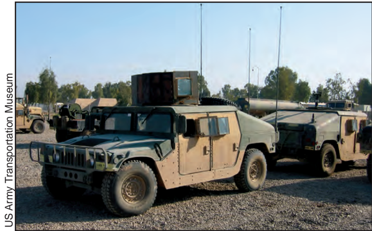
Figure 130. HMMWV M998 gun truck with level 2 ring mount 7.
