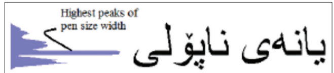
Figure 2. Baseline found with pen-size and row projections. Note that the highest peak is the baseline of a horizontally straight text line
