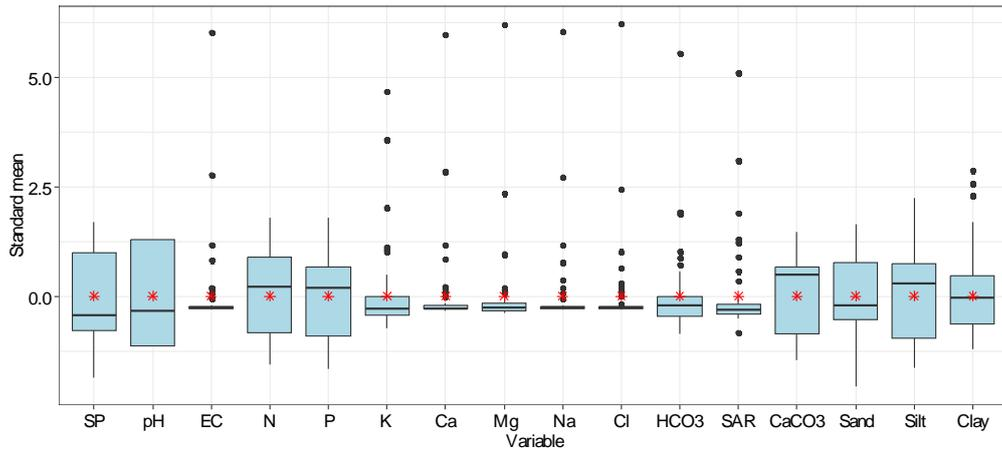
**Fig. 4.** Boxplot with the variables with the standardized data for the soil properties data set in the study area
