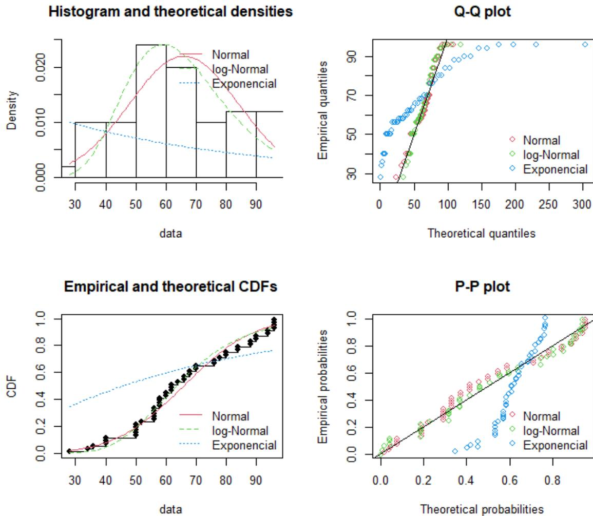
**Fig. 7.** Plot of empirical and theoretical distributions for sand. The density plot or histogram plot in the top-left corner, quantile-quantile (Q-Q) plot or probability plot in the top-right corner, cumulative distribution function plot (CDF) in the bottom-left corner, and probability-probability (P-P) plot in the bottom-right corner.
