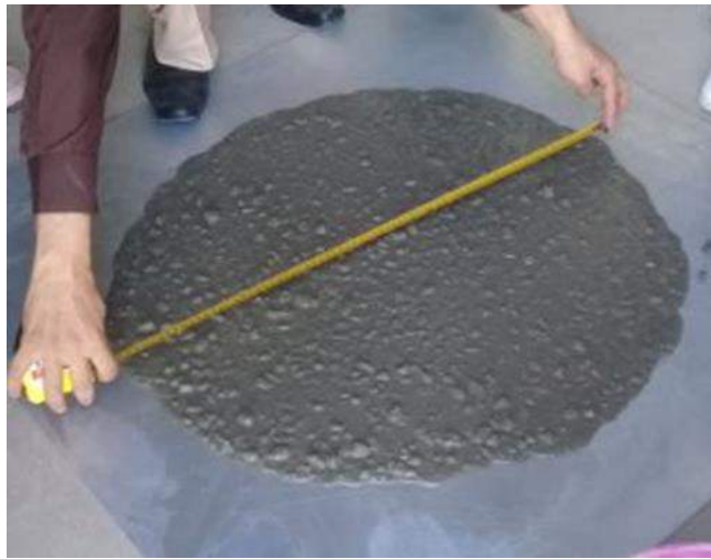
Figure 2.5 Slump flow test
