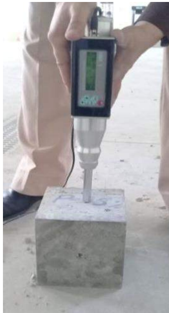
Figure 2.9 Rebound hammer test
