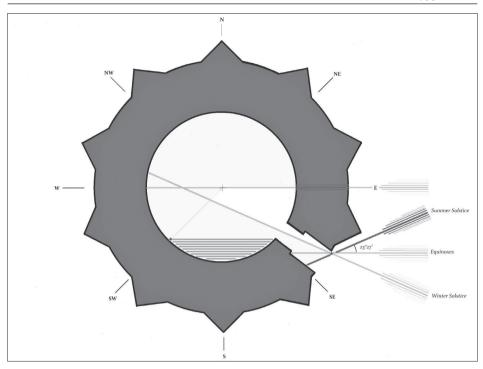
Figure 7. Projection of the sunbeams at sunrise at equinoxes and solstices through the entrance of the Gonbad-e Kāvus tower
